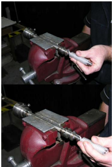
5) Gently twist the heater to and fro while sliding it off the sheath.
