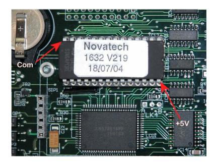
There are spare conductors in the ribbon cable that can be utilised for the 5V rail and the common of the power supply. Solder two jumpers to each of the headers as shown below.
