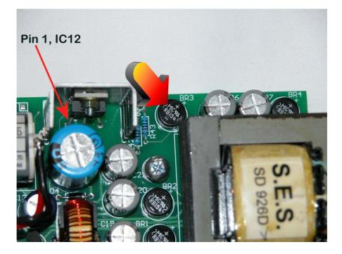
3) On analysers with version 1.6 or earlier 1630-2 boards, the 40-way ribbon cable is worn or damaged. Measure the 5V rail on the 1630-2 PSU board and then on the 1630-1 board. If the value measured on the 1630-1 board is less than the value measured on the 1630-2 then the ribbon cable is causing excessive voltage drop.
