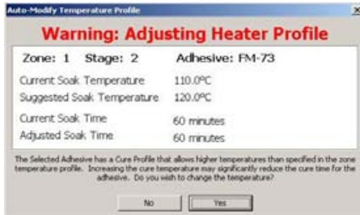
**Fig. 11 Start cycle screen, Automatic Adhesive Selection Parameters**
