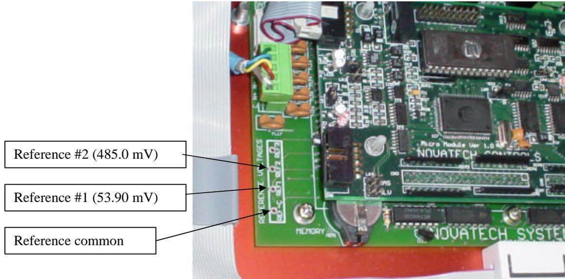
**Fig. 3 HBC-4300-1 Main PCB reference voltages**
