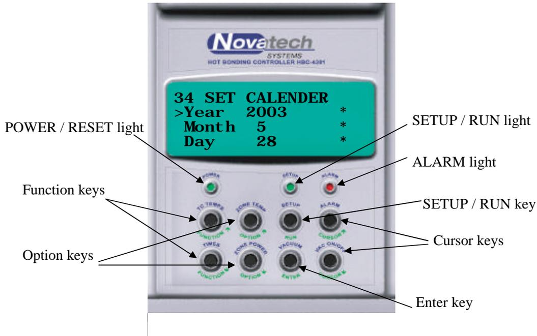
**Fig. 1 HBC-4301 Control case keypad and display**
