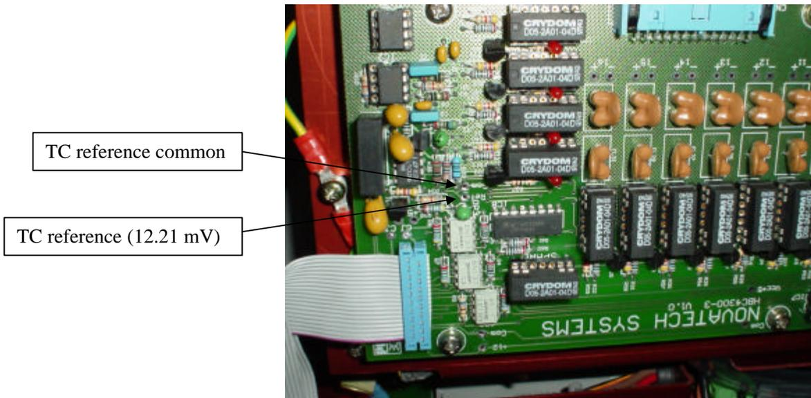
Fig. 2 HBC-4300-3 Thermocouple Input PCB as it is mounted in the Control Case
