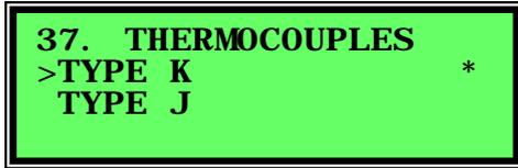
The **cursor** keys or the **option** keys will move the cursor between the two-thermocouple types. The **enter** key will put the asterisk at the end of the line and save the thermocouple type in the BBRAM.
