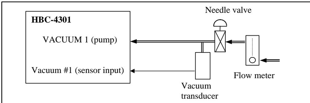
**Fig. 4 Vacuum pump pumping rate test**
