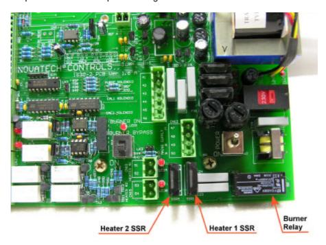
The most common mode of failure for a solid state relay is a short circuit. This will result in 100% power applied to the probe or sensor's heater that will destroy the heater due to excessive temperature.
