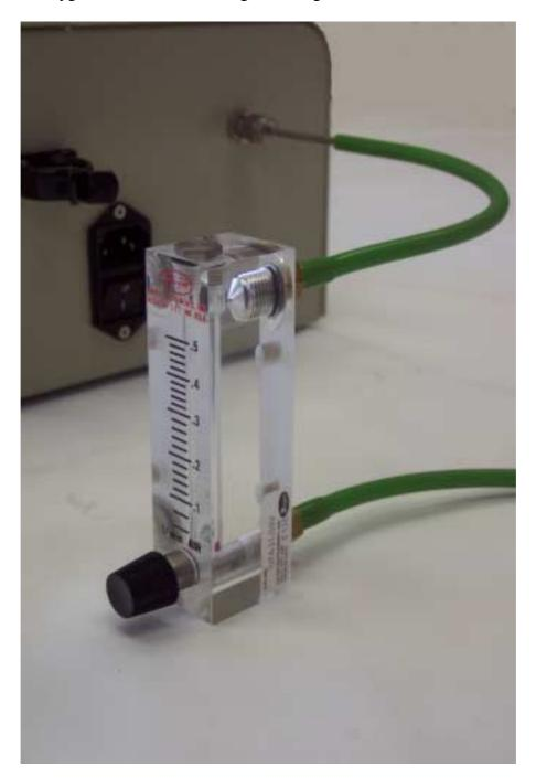
The rotameter is also a useful tool for trouble shooting an analyser. Checking the gas flow rate is a primary test for any analyser that that has response time problems.
