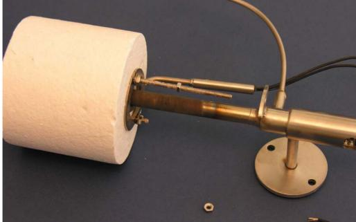
2.4 Slide the heater from the sensor assembly.
