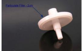
3) The filter has been pushed onto the Luhr fitting on the sample line too hard causing it to split allowing ambient air to dilute the sampled gas. Solution: Replace the filter
